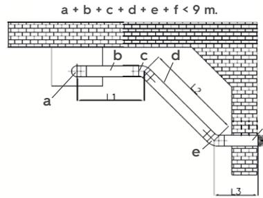
Figure 23 III. Example of flue installation with one 90° bend and two 45° bends
