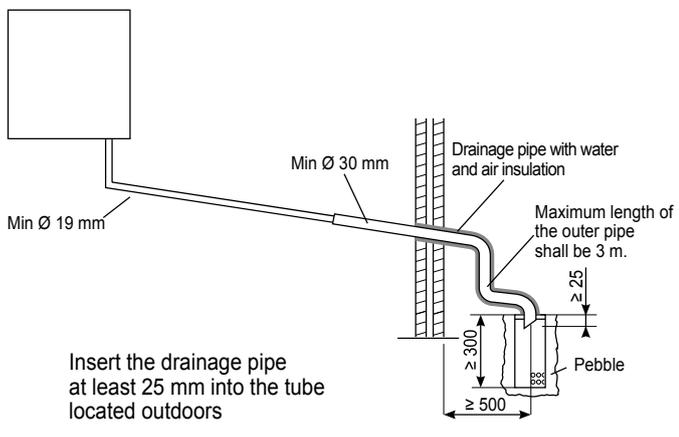
**Figure 32** Outside Connection of Condensate Water Drainage Pipe
