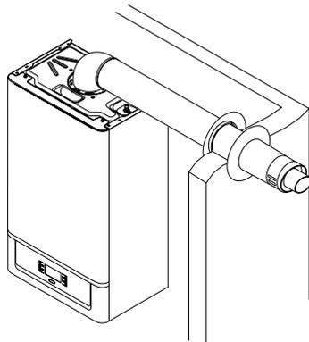
Figure 19 Boiler concentric wall outlet for hermetic use
