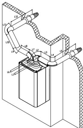
Şekil 26 Example of Split Flue (Hermetic) Type
