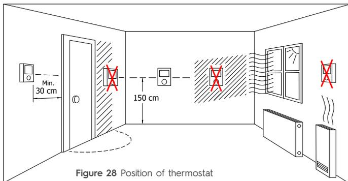
Figure 28 Position of thermostat
