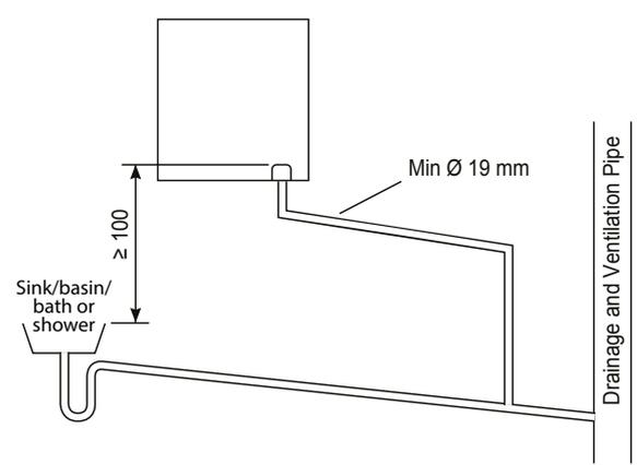
**Figure 31** Connection of Condensate Water Drainage Pipe at Indoor Bathroom Drainage Lower Level
