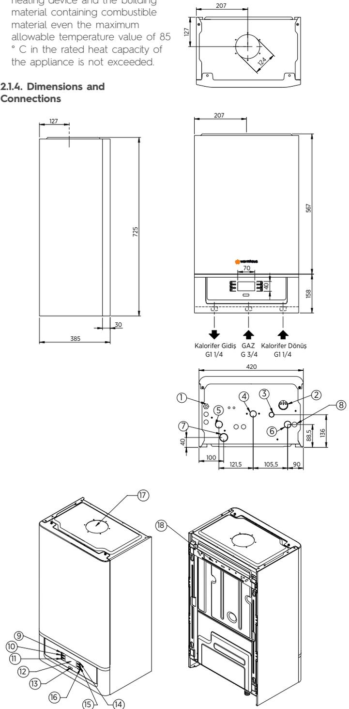
Figure 6 Viwa 50 / Viwa 65 boiler dimensions and connections
