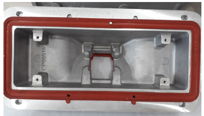
Figure 5.9 Check if there is any damage signs in the impermeability gaskets of burner cover. Change when necessary
