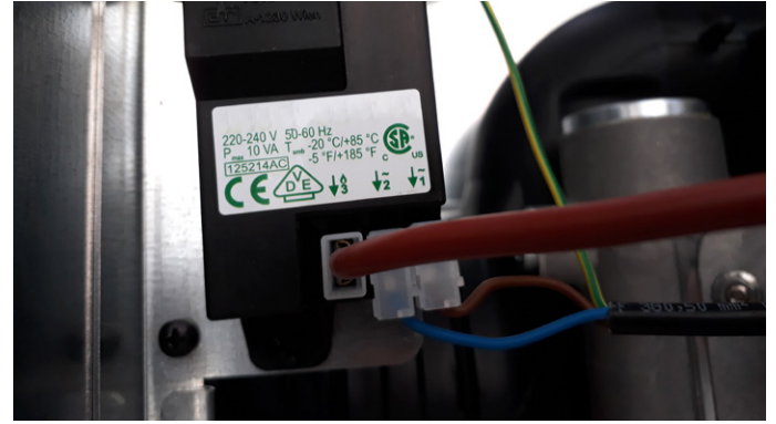
Figure 5.6 Remove the ionized cable coming from Ignition Transformer from ignition electrode.
