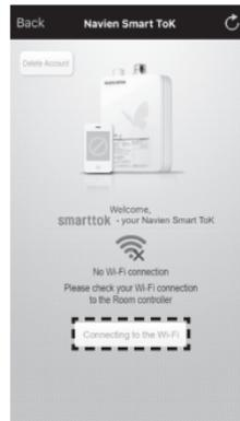
Register the Room Controller to Wireless Router through the Router Connection.
