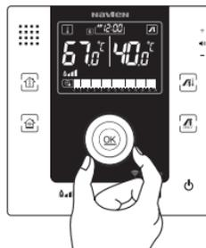
Press OK button to save or leave it as it is after selecting the temperature for auto-save. Temperature control range is 40~90°C at intervals of 1°C. The operation display will appear while the time zone is set to " ON " in the 24 Hour program depending on the set temperature and heating will start.
