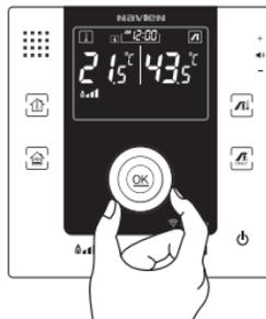
Press OK button after setting the hot water temperature or leave it as it is for auto-save.
