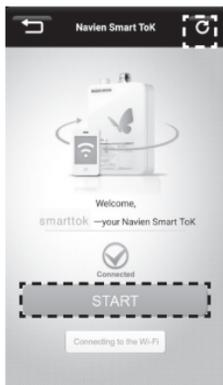
After connecting to router, Check the connection by pressing the 'Refresh' button.
