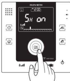
OFF will change to ON if you press OK button and '■' sign will appear on the Timer bar on the bottom. Turn the dial to set the next time you wish to heat then press OK button to confirm.
