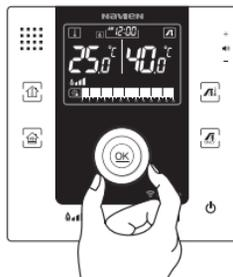
Press OK button to save or leave it as it is after selecting the temperature for auto-save. Temperature control range is 10~40°C at intervals of 0.5°C. The operation display will switch on and heating will start if the current room temperature is lower than the set temperature while the time zone is set to "ON" in the 24 Hour program.
