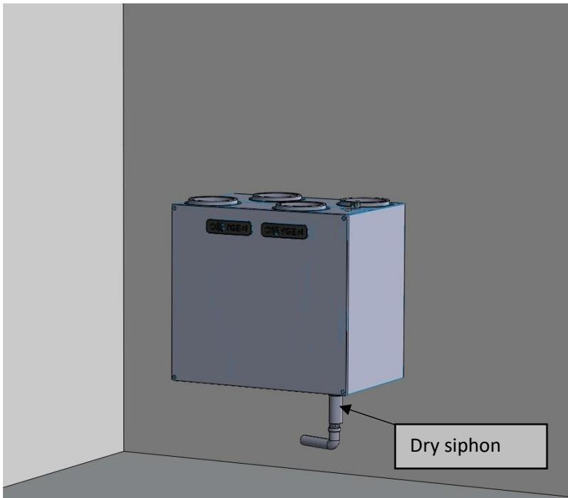
For draining condensate into the sewer, it is recommended to use dry-type siphons:
