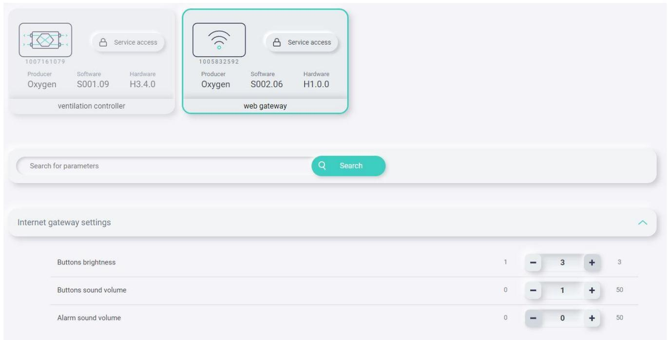
**Ventilation controller** the user menu list that appears in the Controller window allows you to view detailed information about the device and to perform important configuration steps. A detailed description of the user menu
